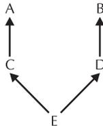
This graph states that class E is derived from both C and D. (That is, that E has multiple base classes, called C and D.) Further, C is derived from A, and D is derived from B.
