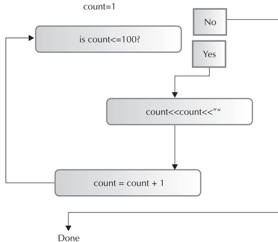
How the **for** loop works.
